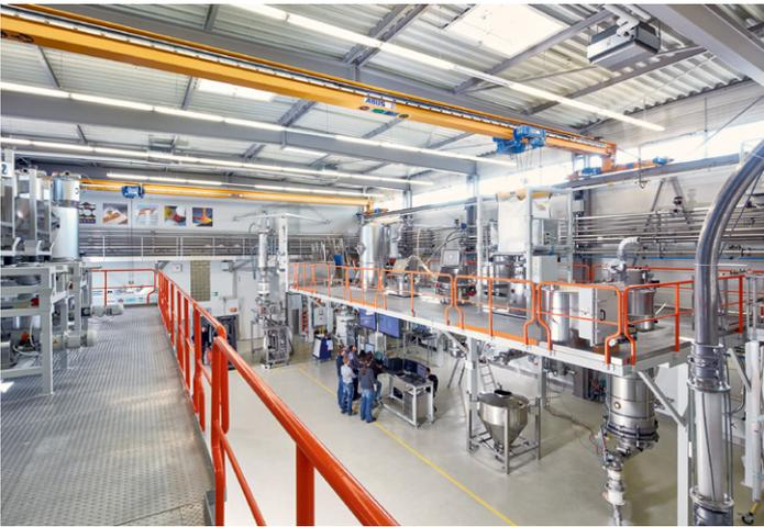
Figure 21: Pneumatic bulk goods conveyor in the development center of AZO GmbH + Co. KG.
